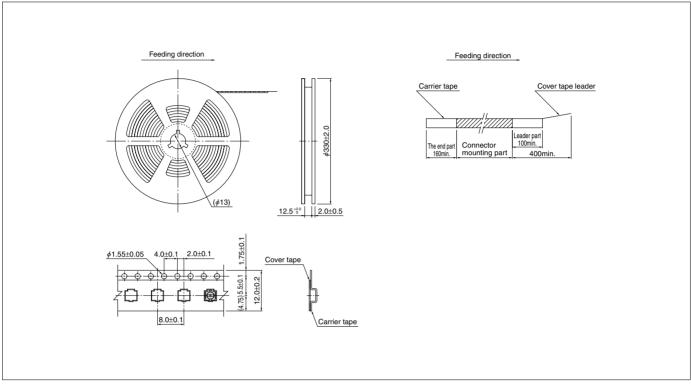
Note: 1. Specifications conform to JIS C 0806. The tape width, connector loading recess square hole dimensions, etc. are determined by the number of circuits and external shape of the connector to be loaded.
