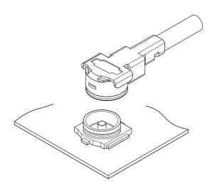
Miniaturized coaxial connector that responds to miniaturized telecommunications apparatus.
