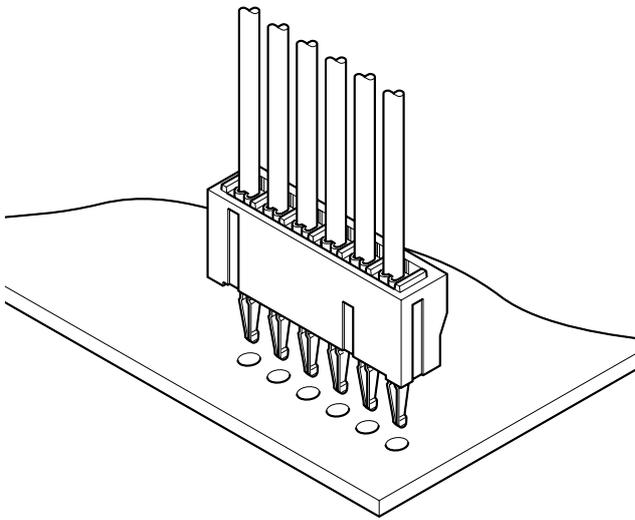
**This low-profile, board-in connector, with a mounting height of only 4.25mm and a thickness of 2.4mm, is soldered directly onto printed circuit boards. The solder tail of the contact is resilient for easy assembly. The housing lances facilitate insertion of contacts.**
