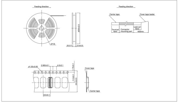
Note: 1. Specifications conform to JIS C 0806. The tape width, connector loading recess square hole dimensions, etc. are determined by the number of circuits and external shape of the connector to be loaded.
