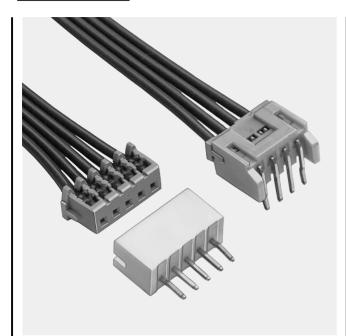
The CR 2.0mm insulation displacement connector features a mounting height as low as 6.9mm and a thickness as thin as 4.8mm (for top entry type). It's suitable for interconnection of UL1007 electric wires in a wide range of electrical and electronic equipment such as VCRs and video cameras.
