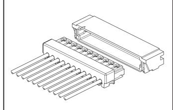
This is the world's smallest 0.6mm pitch ID connector for discrete wires. This Wire to Board miniaturized connector has a mounting height of 1.45mm and depth of 3.0mm.
