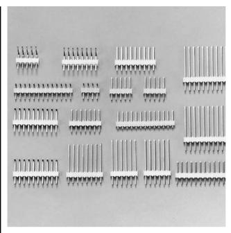
The SB headers can be used to connect any 2.5mm receptacles to printed circuit boards. They can also be used to directly connect PC boards. They come in pitches of 2.5mm and in both top entry and side entry type models.
