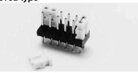
This is a two-circuit jumper connector suited for changing or switching circuits on printed circuit boards without using DIP switches. It is compact and light, thus can be mounted on printed circuit boards without interfering with the placement of other components. The connector is easy to use, low in cost, and has a wide range of applications in industrial and consumer products.
