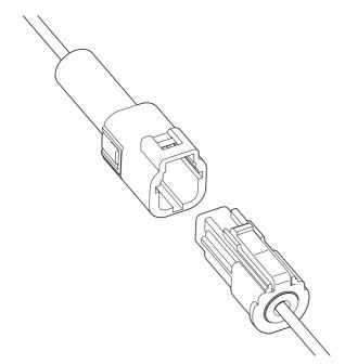
This connector is compact and excels in waterproof and durability. This wire-to-wire connector can be used for the place of which especially waterproof is required. Its waterproof grade is 7 ingress protection of JIS C 0920 (IEC 60529 IPX7).
